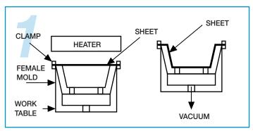
Straight vacuum forming in a female mold is recommended for low-profile parts where deep draw is not a requirement.
