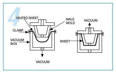
Vacuum forming with snap-back can reduce starting sheet size, aid material distribution, and minimize chill marks.
