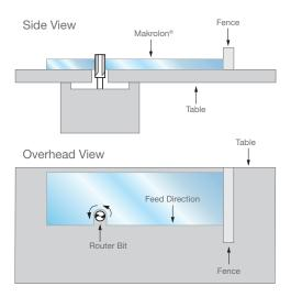
It is important to feed the sheet against the rotation of the router bit and to provide a fence for sizing when making straight cuts.
