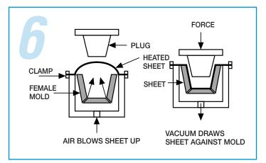
Forming with billow plug is often used to produce thin-wall items with depth-to-diameter draw ratios up to 1.5:1.
