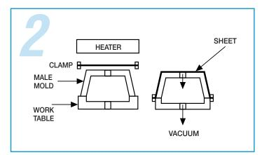
Drape forming over a male mold usually results in better material distribution and depth-to-diameter draw ratios.
