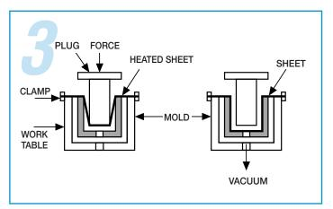
Thinning of material in deep-mold cavities can be overcome by use of plug assists designed for fast penetration.
