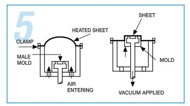
Air-slip forming is similar to vacuum snap-back except that heated sheet is billowed up and mold rises to meet it.
